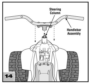
• Fit the handlebar assembly onto the end of the steering column. Make sure the handlebar grip area points towards the rear of the vehicle.
